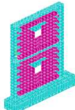
Fig. 7.d. Typical meshing (Windows Opening)
