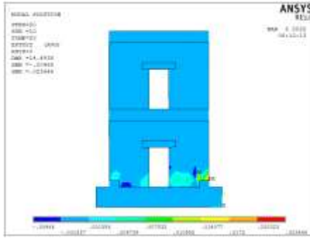
Fig 21.g. Mechanical strain at failure load - (front elevation) Model (S-02-FEM-M).
