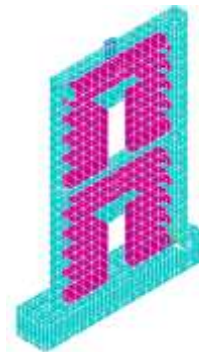
Fig. 7.c. Typical meshing (Doors opening)
